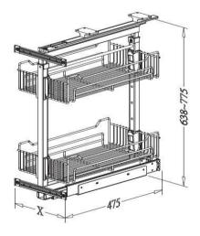
Adjustable Height of 638mm - 775mm Soft Closing Runners 50kg Loading Capacity 300mm Cabinet Unit Basket Sizes 250mm x 460mm 400mm Cabinet Unit Basket Sizes 345mm x 460mm
