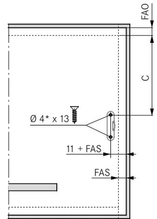
\* Pre-drilling required - Ø 2 mm
