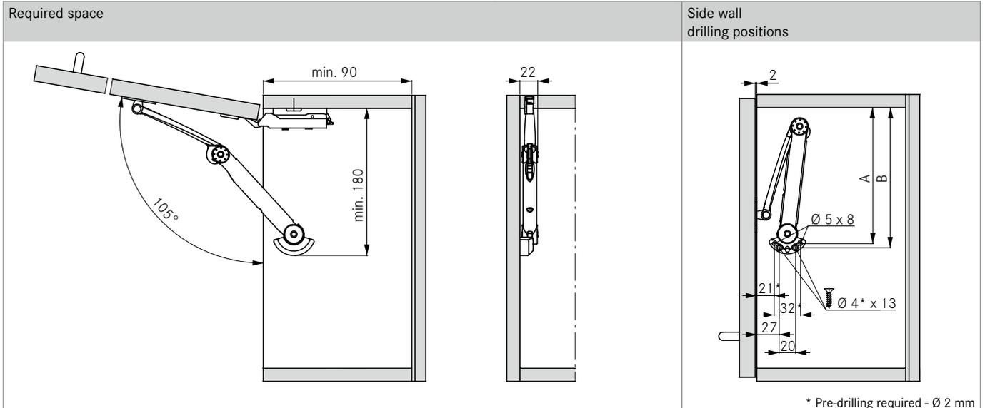
\* Pre-drilling required - Ø 2 mm
