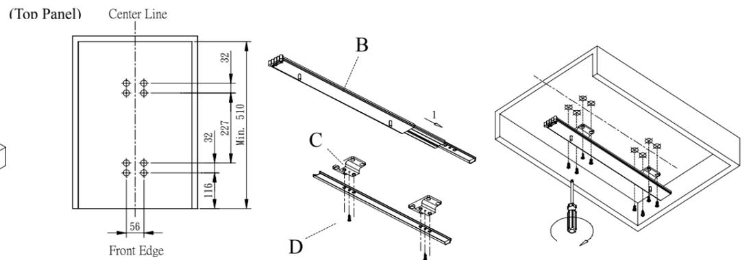
STEP 3: 1: Keeping the frame in the closed position, fasten the frame to bottom runner using enclosed screws (F) and washers (G).
