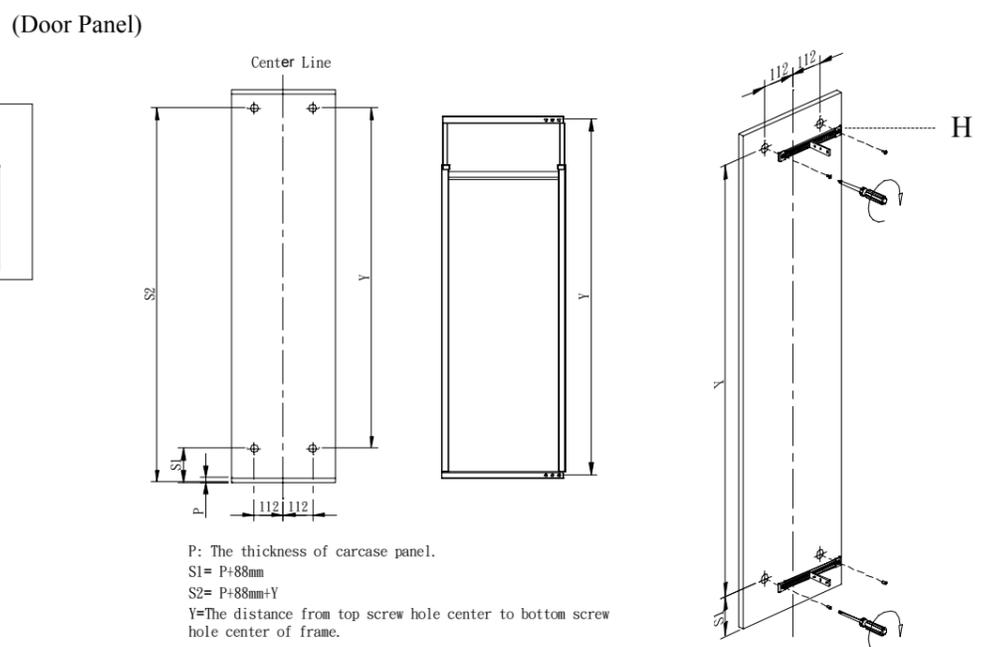
STEP 5: 1: Release middle screw of T-Bar, push together T-Bar to frame tubing, then tighten the middle screw and two screws on T-Bar.
