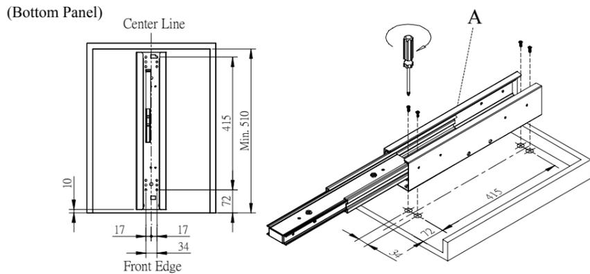
STEP 2: 1: Mark center line on top panel and screw hole positions for plastic base (C) of top slide (B).
