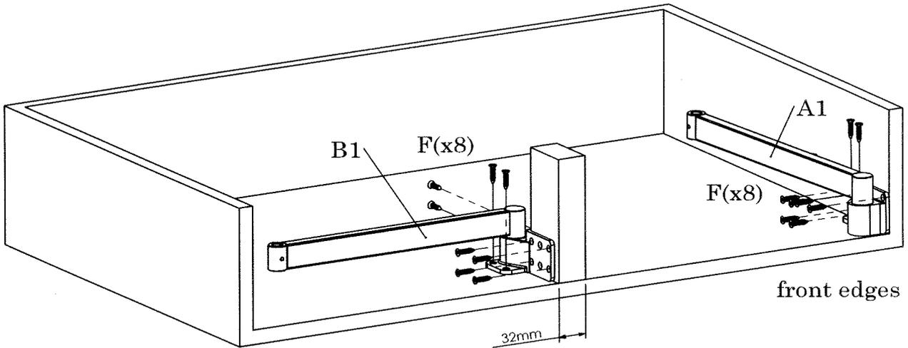
step 2: install Internal Swing Arm (B2) and External Swing Arm (A2) with Screw (F). Align External Swing Arm (A2) with side board edges.
