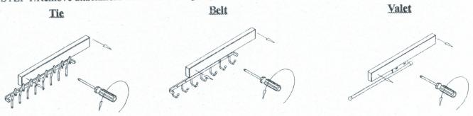
STEP 2: Mount slide base using 2 euro-screws provided, then connect the housing to slide.
