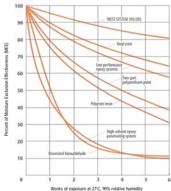
Adding solvent compromises the moisture resistance of cured epoxy
